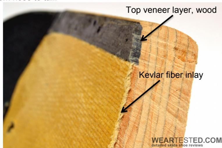
The remaining 6 veneer layers are said to be slightly thinner, but the overall construction is still a 7-ply deck. Apart from being supposedly lighter and thinner than other decks, other positive aspects of the construction are the improved distribution of stress along the deck and a faster and higher rebound, according to the manufacturer. The latter is said to increase what skateboarders colloquially call “pop”.
