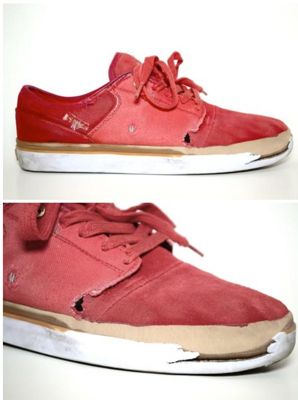
This special colorway features a canvas sidewall, which is more prone to abrasion than suede. As a result the meeting point of the toebox- and the sidewall panel turned out to be a weak spot: There's a hole and the black inner material is visible.
