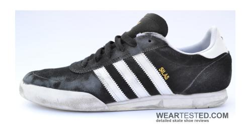
The fine pattern of the sole, usually a weak spot, showed no wear-out spots during our 10h test. But, when the model was skated longer, they showed up, hinting at a possible weakness of the Silas SLR. Also, the mesh inner part in the heel area of the shoe is prone to abrasion by griptape contact.
